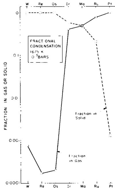
Fig. 7. The calculated composition of an "ultra"-refractory metal alloy produced by fractional condensation at 1675 K and  $10^{-3}$  bars. The metals remaining in the gas condense to form an Ir-Mo-Ru alloy. Neither pattern matches the observed Mo and W depletions.
