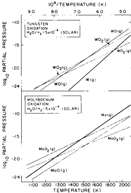
Fig. 2. Gas chemistry over solid W and solid Mo. W is more easily oxidized than Mo and is also more refractory. The results are for the canonical solar nebula oxygen fugacity.
