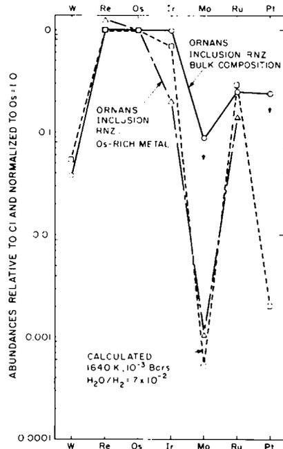
Fig. 3. Observed and calculated refractory metal abundances in Ormans inclusion RNZ [5]. The bulk composition (see Table 1) is from neutron activation; the Os-rich metal composition is from electron microprobe analysis.
