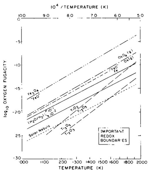
Fig. 9. Oxygen fugacity buffers for several Ti and Fe oxides compared to the canonical solar nebula oxygen fugacity. Oxygen fugacities corresponding to higher ( $\text{H}_2\text{O}/\text{H}_2$ ) ratios are also shown. The line where 50% of all Os gases are present as  $\text{OsO}_4(\text{g})$  is also shown.
