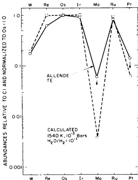
Fig. 5. Observed and calculated refractory metal abundances in the Allende FUN inclusion TE [13,14]. The bulk composition from neutron activation is in Table 1.
