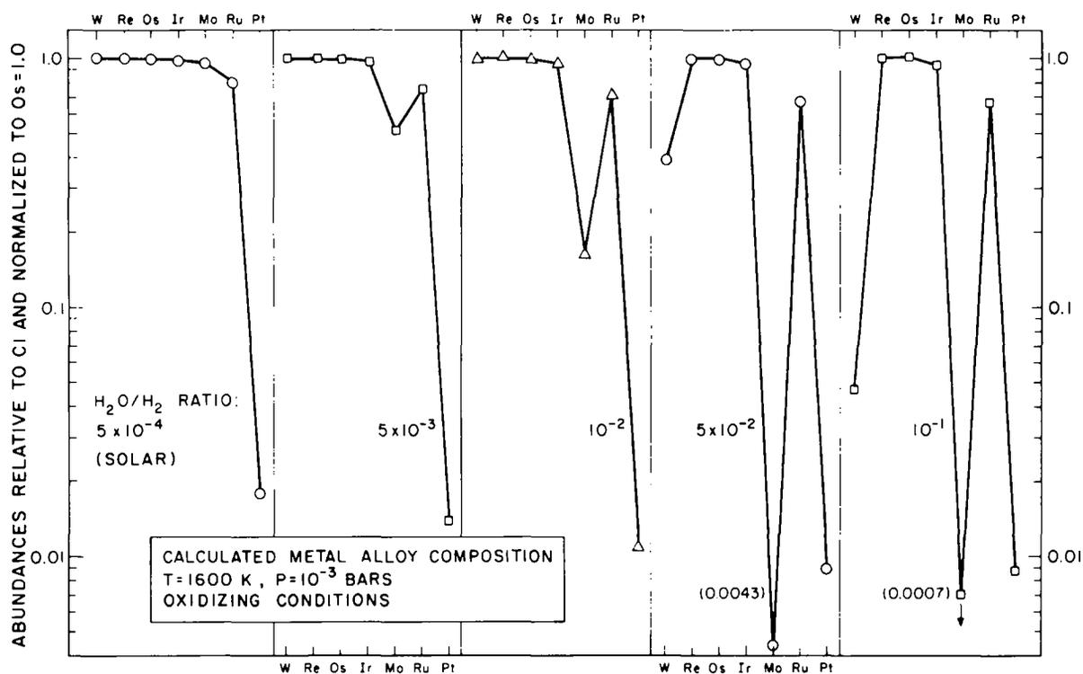
Fig. 1. Mo and W depletions in refractory metal alloys as a function of oxygen fugacity at constant temperature and pressure. The oxygen fugacity is expressed as the  $(\text{H}_2\text{O}/\text{H}_2)$  ratio, and can be calculated from  $\log_{10} K(\text{H}_2\text{O}, \text{g})$  in JANAF [22].
