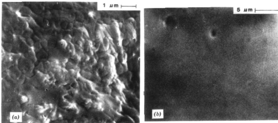
**Figure 26.11** SEM of B-doped SiO<sub>2</sub> particles coated with boric acid and NaCl and sintered at 1050°C for 2 hr: (a) top surface and (b) fracture surface.
