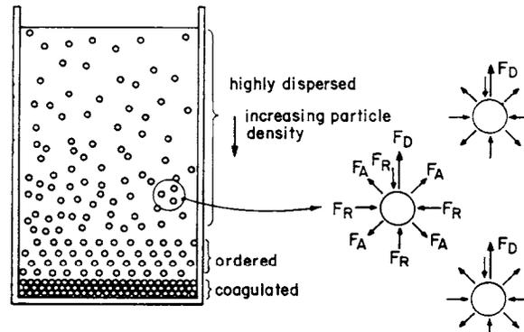
**Figure 26.2** Schematic representation of the ordering of monosized particulates from a liquid phase caused by equal drag forces,  $F_D$ , and isotropic and equal electrostatic repulsion,  $F_R$ , and van der Waals attraction,  $F_A$ .
