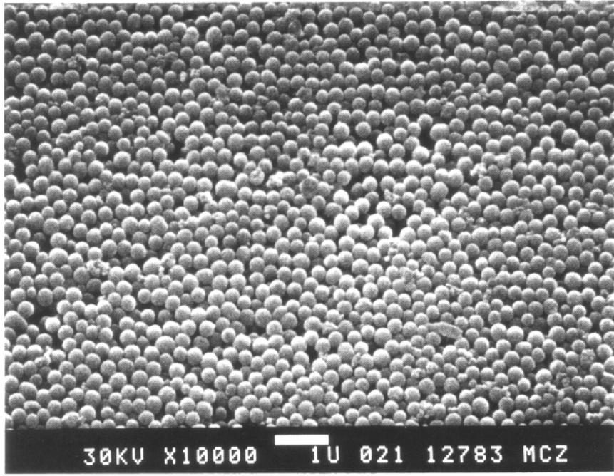
**Figure 26.12** Top surface of a compact of Ba-Nb-doped TiO<sub>2</sub> (0.2% BaO and 0.5% Nb<sub>2</sub>O<sub>5</sub>).
