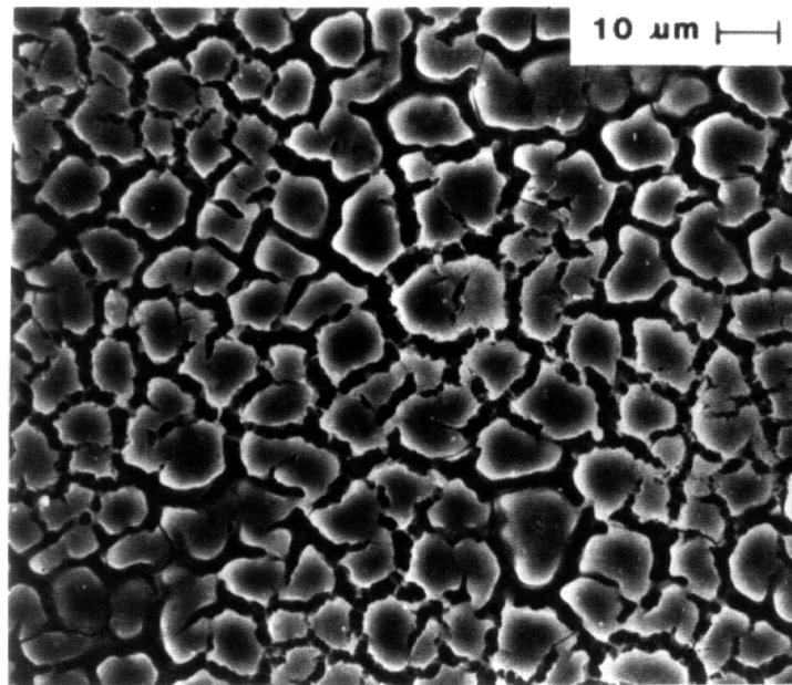
Figure 26.9 SEM of a  $5 \mu\text{m}$  film of B-doped  $\text{SiO}_2$  particles sintered at  $1000^\circ\text{C}$  for 5 hr.
