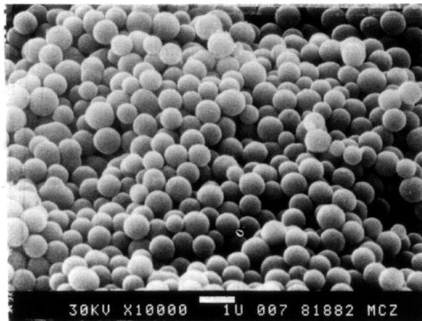
**Figure 26.4** Fracture surface of a compact of Sr-Ta-doped TiO<sub>2</sub> ( wt. % SrO and 1 wt. % Ta<sub>2</sub>O<sub>5</sub>).
