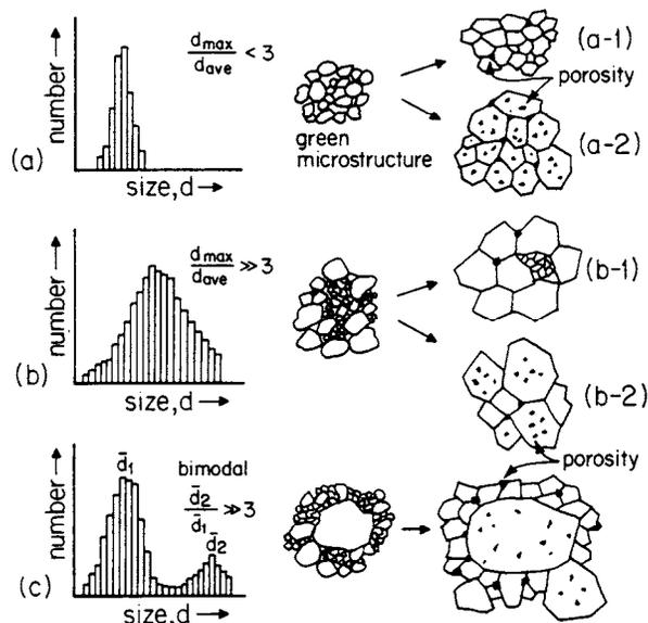
**Figure 26.1** Schematic representation of the effects of powder size distribution on the sintered microstructure. For example, in (a-1), with a narrow size distribution and control of the grain boundary-pore interaction, dense sintered ceramics with the grain size slightly larger than the particle size are possible.
