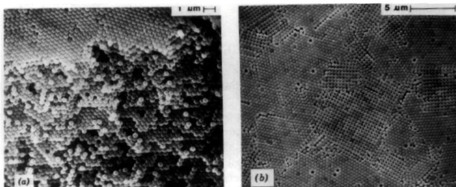
Figure 26.3 Fracture (a) and top (b) surfaces of a compact formed from monodisperse boron-doped  $SiO_2$ .
