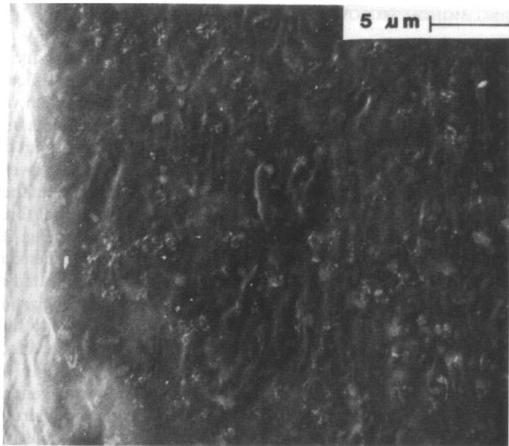
**Figure 26.10** SEM showing the surface of a thin cake of B-doped SiO<sub>2</sub> sintered at 1000°C for 1 hr.
