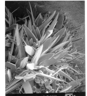
Magnetite growth on Fe-Ni metal
